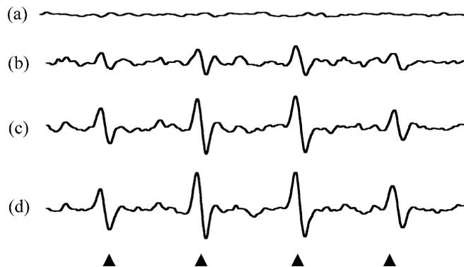
**Fig. 1** EPR spectra of DMPO–OH spin adduct (assigned by *triangle*), attributed to  $\cdot\text{OH}$  radicals formation in 0.5-mg/ml collagen illuminated with 40-mW/cm<sup>2</sup> broadband visible light: **a** control, **b** 10 min of illumination (24 J/cm<sup>2</sup>), **c** 20 min of illumination (48 J/cm<sup>2</sup>), **d** 30 min of illumination (72 J/cm<sup>2</sup>)
